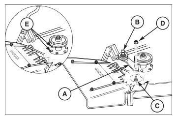
Figure 9. Install Idler Assembly
